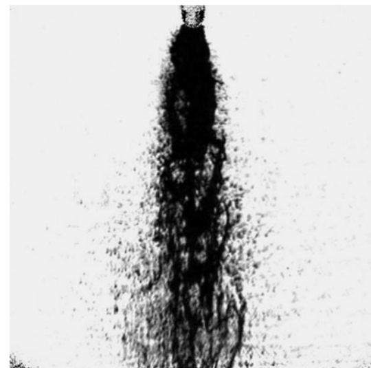
Fig. 8 Ballistic image of flow case 8 described in Table 1: Q_L = 0.53 (L/min), GLR = 1.43
