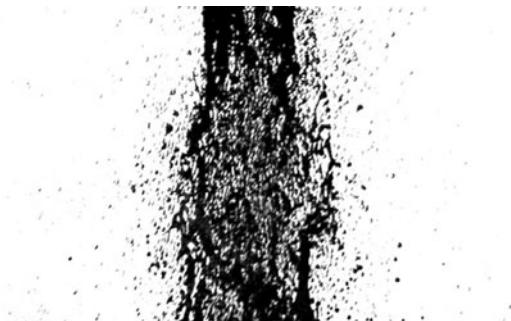
Fig. 3 Ballistic image of an aerated spray with Q_L = 0.67 (L/m) and GLR = 2
