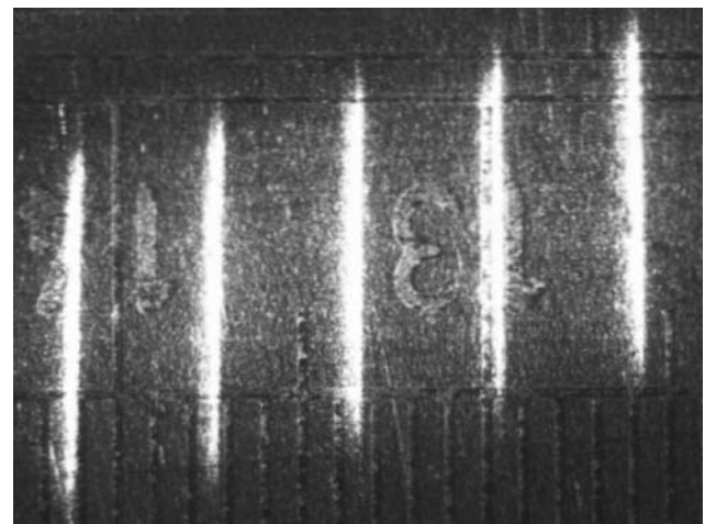
Fig. 2 Intensity distribution of five scanning light sheets on a metal scale with an inclined angle of 19^\circ
