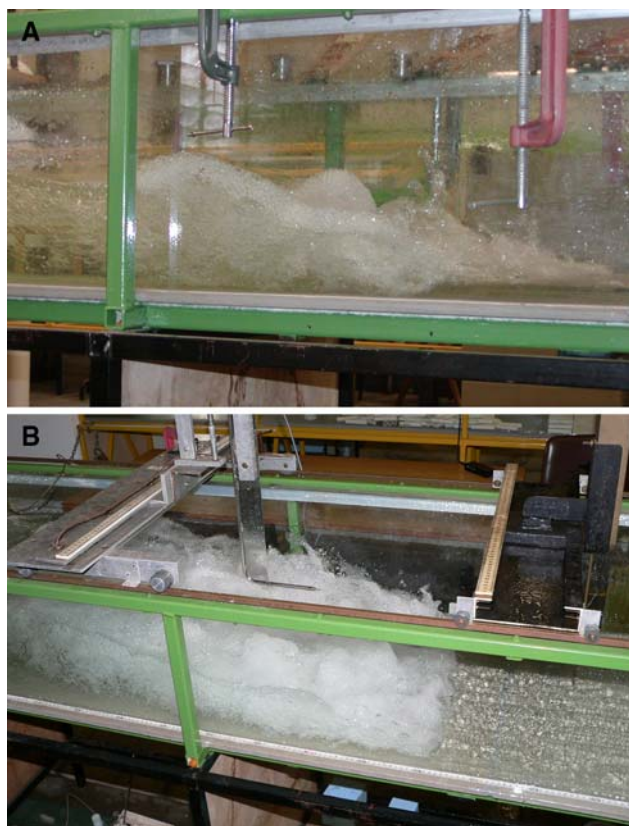
Fig. 2 Bubble entrainment in hydraulic jumps. a Fr_1 = 5 , Re = 38,000 , x_1 = 0.75 m, d_1 = 0.018 m, shutter speed: 1/40 s, flow from right to left. b Fr_1 = 8.3 , Re = 62,000 , x_1 = 0.75 m, d_1 = 0.018 m, shutter speed: 1/80 s, flow from right to left. The phase-detection probe is visible above the recirculation region
