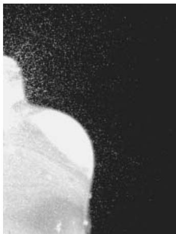
Fig. 5. Typical feature of the atomizing results for high voltage where the big cone and a fine cloud of droplets are observed. In this case, the image was obtained recording the laser-induced fluorescence signal of sulforhodamine seeded in the atomized water. The resolution is 5 \mu\text{m}/\text{pixel} , a field of view of 1.45 \times 1.9 \text{ mm} , zone b in Fig. 2, and an excitation voltage of 33 V
