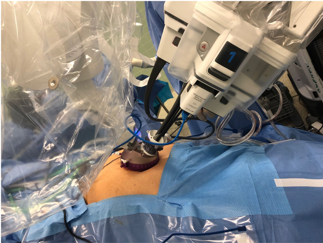
Fig. 1 da Vinci SP single robotic arm with multiple instruments entering through a single port
