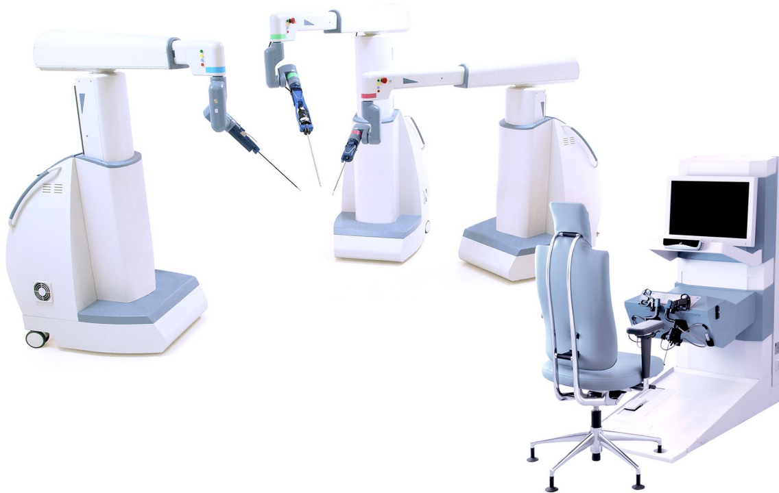
Fig. 1 The Senhance Surgical Robot seen here with three arms and the cockpit/open console
