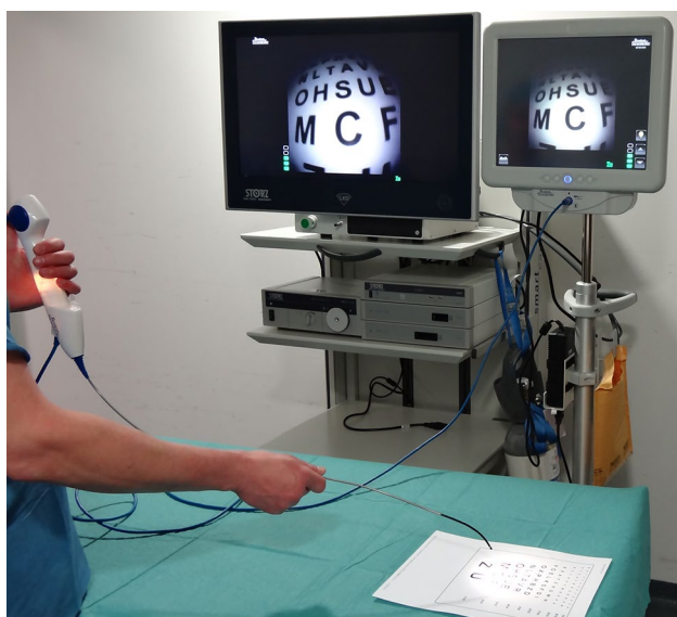
Fig. 3 LithoVue™ connected via its cable to the all-in-one touchscreen computer including monitor workstation (right) and image processing software and simultaneously connected to the operating room's monitor (left) via a DVI connection
