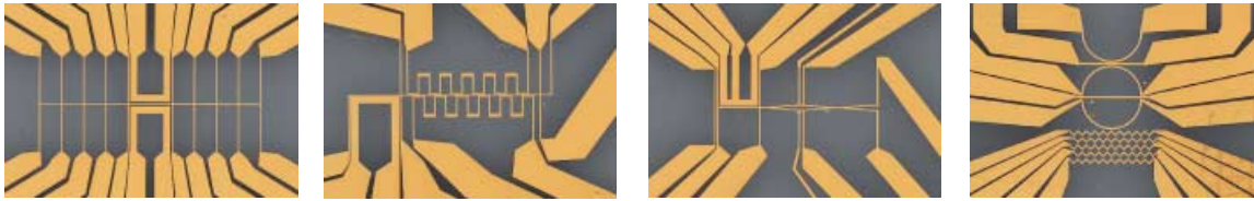
FIGURE 20 Photographs of various chip trap substrates (gold on AlN, original size 10.7 mm × 7.1 mm each). From left to right : quadrupole traps and Ioffe–Pritchard traps of various aspect ratios; the atomic conveyor belt; guides with electrical field electrodes between Y-shaped splitting and recombining regions; magnetic lattice structure. All four substrates were produced in Munich in 1999; to date, only the first two have been used in experiments
