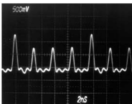
FIGURE 5 Output pulse train of an OPO with a repetition rate of 336 MHz, corresponding to four-times the repetition rate of the pump laser. Note that the cavity length of the OPO is 1339.3 mm. The cavity length difference between the OPO and the pump laser is 446.4 mm, which is one fourth of the cavity length of the pump laser
