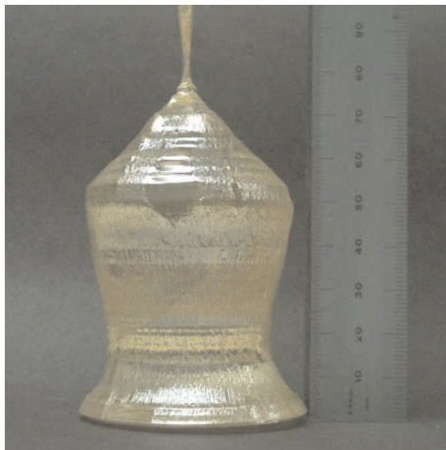
Fig. 1. Photograph of an as-grown boule of Mg-doped nearly stoichiometric \text{LiNbO}_3
