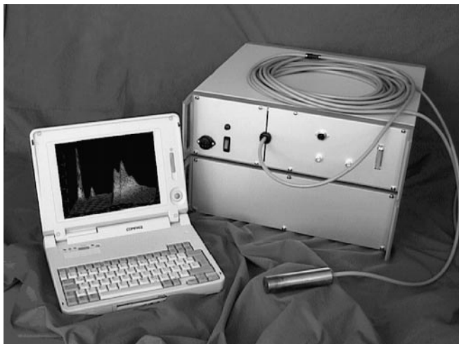
Fig. 1. Photograph of the fiber-optic LIF instrument consisting of two 19" cases containing a pulsed diode-pumped Nd:YAG laser with frequency conversion into the UV, and an optical multichannel analyzer. The system is controlled by a laptop PC via the parallel port. The fiber-optic probe with 15-m-long cable is also shown
