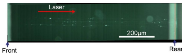
Fig. 13 Damage characteristics of fused silica under a laser fluence of 2.96 J/cm 2
