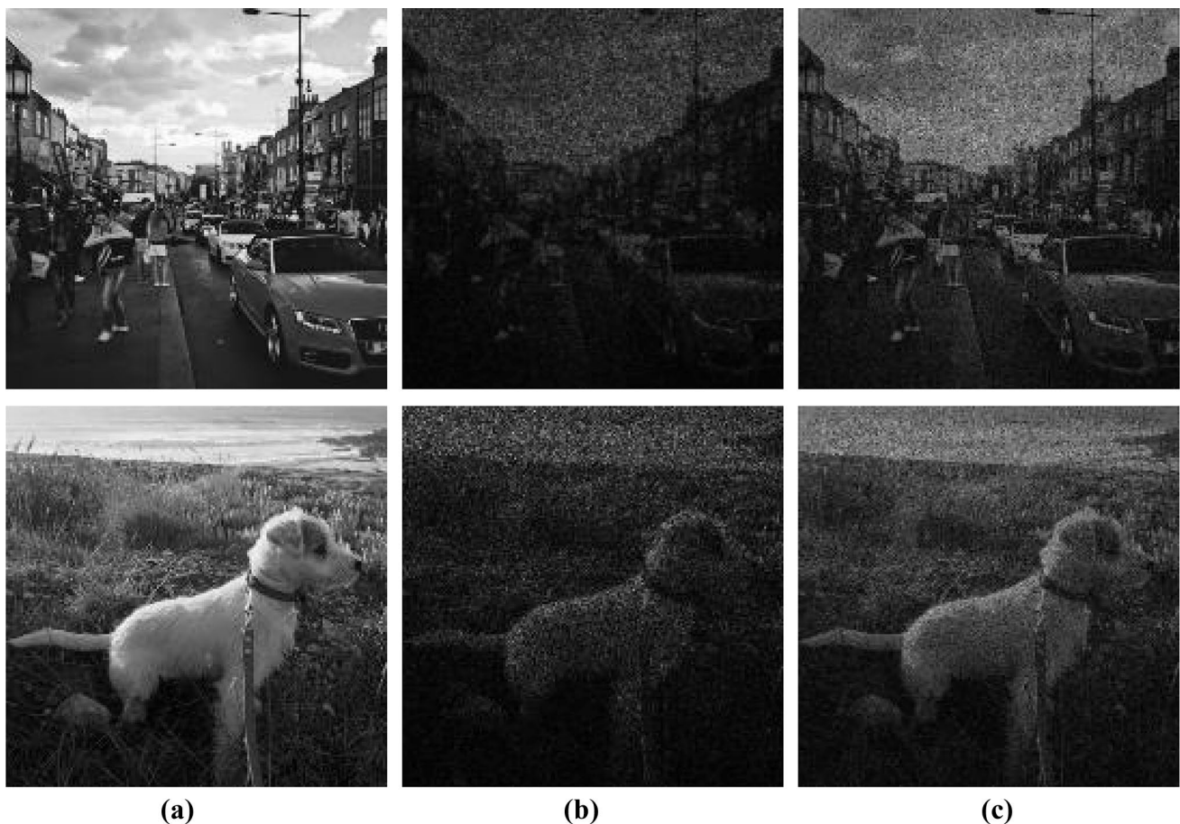
Fig. 1 Original and reconstructed images: a we used two different images as shown in each row, b numerically reconstructed images from phase-only CGHs without the GS optimization with random
