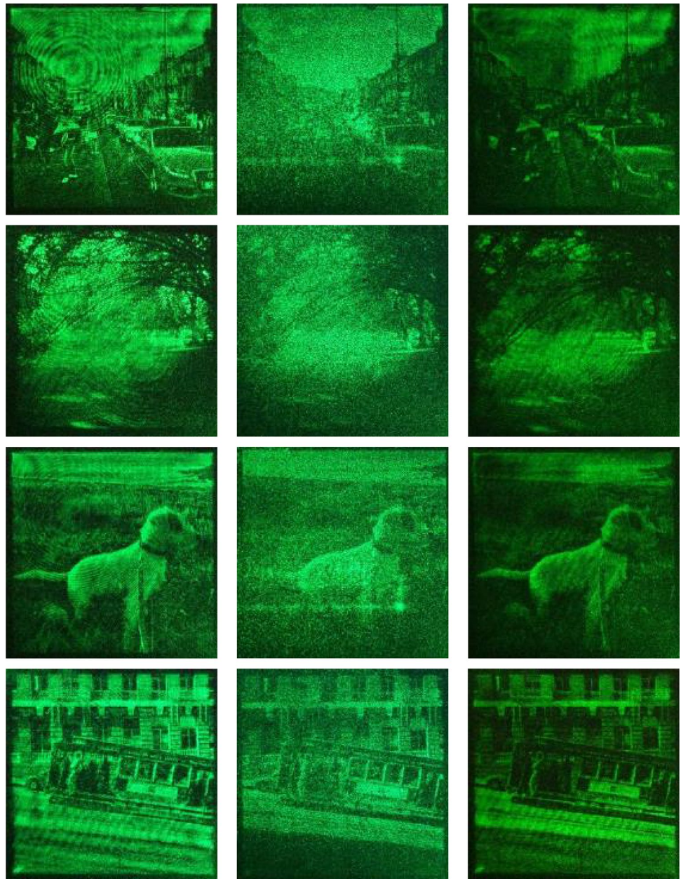
Fig. 8 Optical reconstructed images of the bleached-phase holograms. From left to right, non-optimization, GS algorithm (10 iteration), and the proposed method
