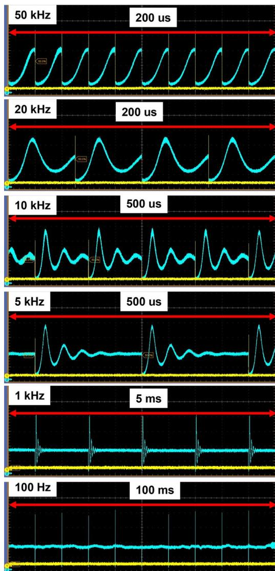
**Fig. 13** Measured time dynamics of intracavity laser power and output pulse for the cavity-dumped Cr:LiSAF at different dumping rates between 100 Hz and 50 kHz. The data were taken at an absorbed pump power of 730 mW using a 0.3% transmitting OC, while using a PC on signal with a length of 15 ns
