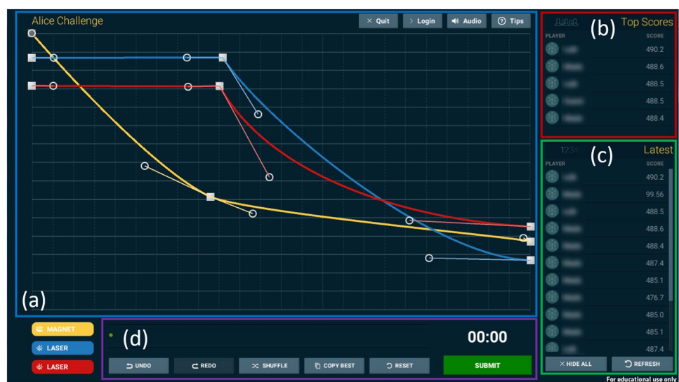
Fig. 2 A screenshot of the interface used in the Alice Challenge , showing a the spline editor used to create the ramps of the laser powers and coil current, shown on a logarithmic scale, b the top score list, c the latest executed sequences, and d the control buttons, including the estimated wait time until the submitted sequence is returned
