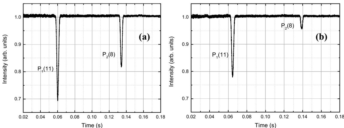
**Fig. 7** Transmission spectra in the absorption section of the HF molecules emitting from the combustor: **a**  $P_1(11)$  and  $P_2(8)$  lines with notable absorption; **b**  $P_2(8)$  line with negligible absorption
