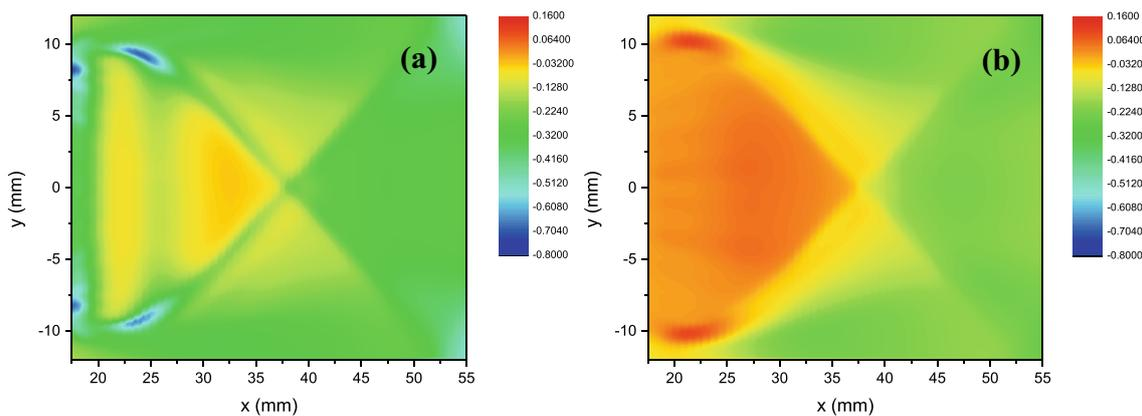
Fig. 2 Calculated small signal gain of HF laser with  $\alpha$  of absorption section ( $\alpha=1.5[\text{NF}_3]/[\text{H}_2]$ ) set to 1.64: **a**  $\text{P}_1(11)$  line; **b**  $\text{P}_2(8)$  line
