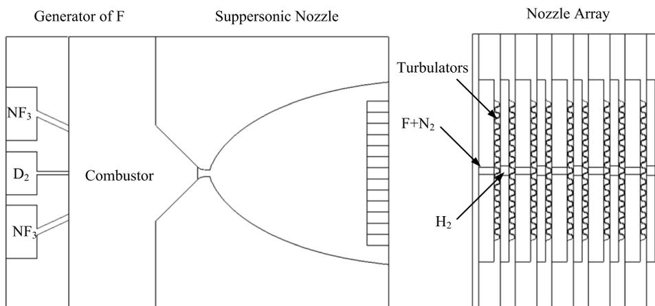
**Fig. 6** Schematic diagram of the experimental setup for obtaining  $P_2(8)$  single line oscillation
