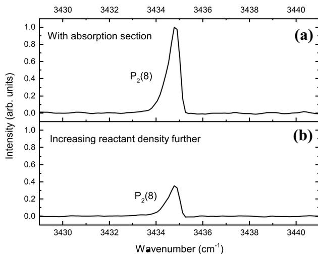
**Fig. 10** Absorption of P<sub>2</sub>(8) line with increasing the flow rate of reactants. **a** Radiation of single P<sub>2</sub>(8) line; **b** decrease of P<sub>2</sub>(8) line as further improving absorption
