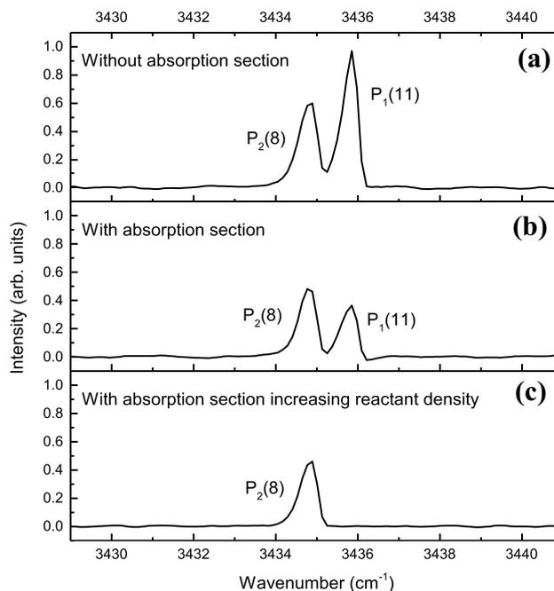
**Fig. 9** Spectra of output laser using fundamental HF particles: **a**  $P_1(11)$  and  $P_2(8)$  lines without absorption; **b**  $P_1(11)$  absorbed by fundamental HF; **c** output of single  $P_2(8)$  line
