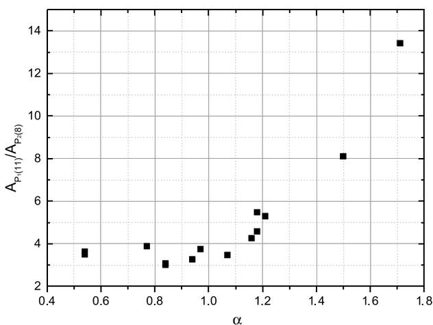
**Fig. 8** The ratio of  $P_1(11)$  line absorbance to  $P_2(8)$  line absorbance as a function of  $\alpha$
