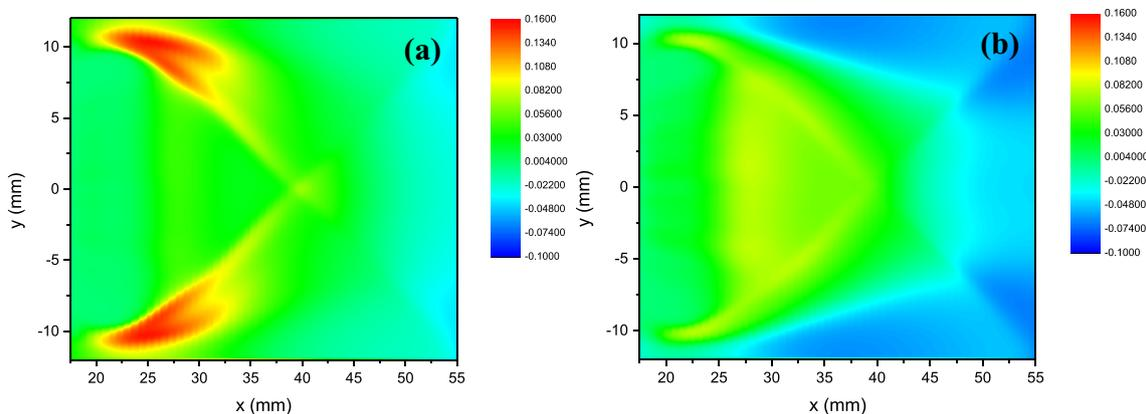
**Fig. 1** Calculated small signal gain of HF laser with  $\alpha(\alpha = 1.5[NF_3]/[D_2])$  set to 1.5 without absorption section: **a**  $P_1(11)$  line; **b**  $P_2(8)$  line
