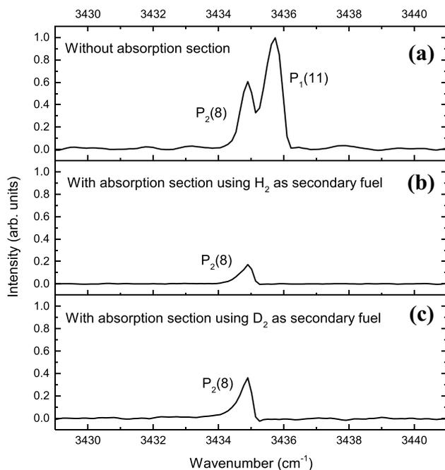
**Fig. 11** Spectra of output laser using D<sub>2</sub> as secondary fuel instead of H<sub>2</sub> to react with F in absorption section. **a** P<sub>1</sub>(11) and P<sub>2</sub>(8) lines without absorption; **b** using H<sub>2</sub> as secondary fuel of absorption section; **c** using D<sub>2</sub> as secondary fuel of absorption section
