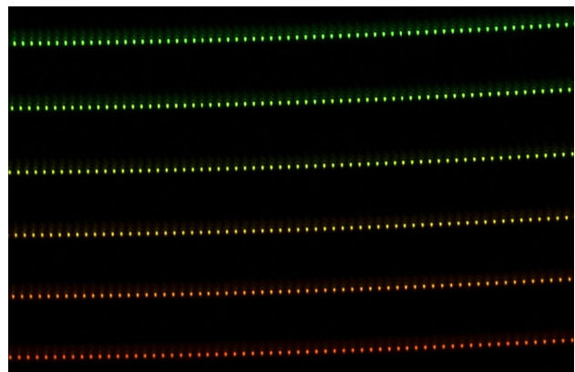
Fig. 4 Part of the echellogram near the center of the image sensor
