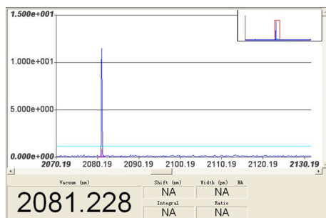
Fig. 4 Spectrum of Ho:YAG laser with SLM operation
