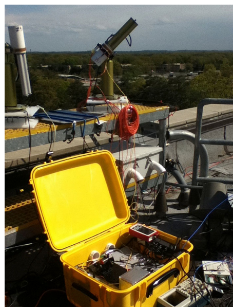
Fig. 3 The mini-LHR (shown housed in a weather-proof case) collects sunlight with fiber-coupled collimation optics connected to an AERONET sun tracker (shown at top of photo)
