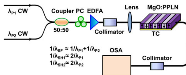
Fig. 2 Type-I QPM SHG and SFG experimental setup
