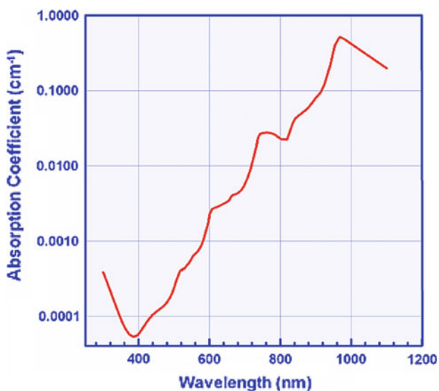
Fig. 2 Wavelength dependence of the water absorption coefficient [22]. The range chosen for the ablation tests was near the minimum at 355 nm
