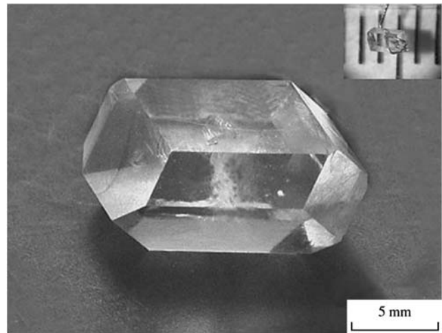
Fig. 2 Er,Yb:YAB single crystal and seed (in the inset)
