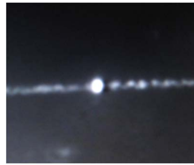
Fig. 6 Output near-field profile from a 1.7 cm long waveguide at 1550 nm. The input signal power is 0.05 mW
