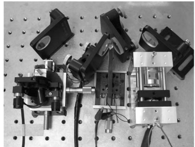
Fig. 8 Photograph of the SPPC ECDL system, paralleling the layout shown in Fig. 7. The laser diode mount (with cover removed to reveal its beam-shaping optics) is in the lower right-hand portion of the photograph, the compact 3-mirror ring-cavity filter (with its relatively bulky micro-positioning control mechanism) is central, and the photorefractive crystal (also micro-positioned) is on the left. The scale is indicated by the 25-mm spacing of tapped holes on the optical breadboard
