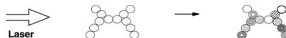
Fig. 2 Illustration of the possible morphological and structural changes that may occur in an aerosol subjected to high-intensity laser radiation such as in LII
