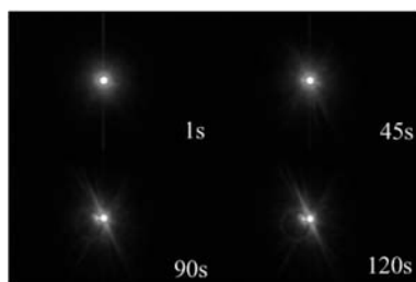
Fig. 2 Temporal evolution of intensity distribution of far-field scattering light
