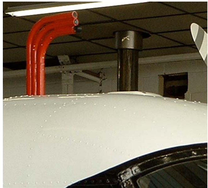
FIGURE 2 The forward facing inlet, mounted on the aircraft roof, is used to sample the atmosphere
