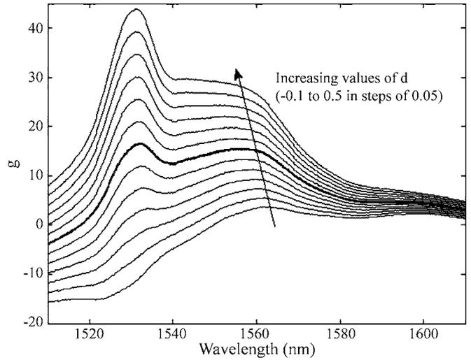
FIGURE 3 Gain coefficient at different wavelengths calculated for different values of average inversion levels in the fiber
