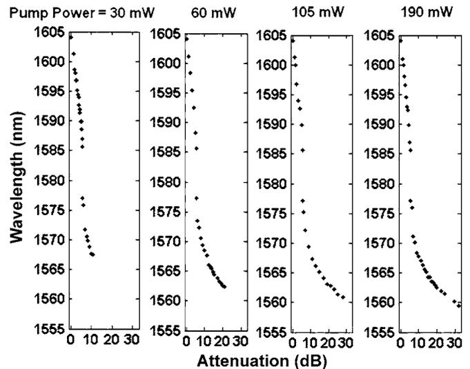
FIGURE 4 Lasing wavelength at different values of  $\alpha$  for different pump powers with  $L = 12$  m,  $R = 0.99$
