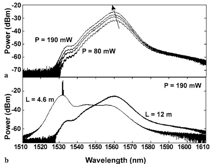
FIGURE 5 (a) ASE spectrum at the output coupler, with a single pass through the EDF for  $L = 12$  m; (b) ASE spectrum for  $L = 12$  m and  $L = 4.6$  m at  $P = 190$  mW. The wavelength scale is identical for both the plots
