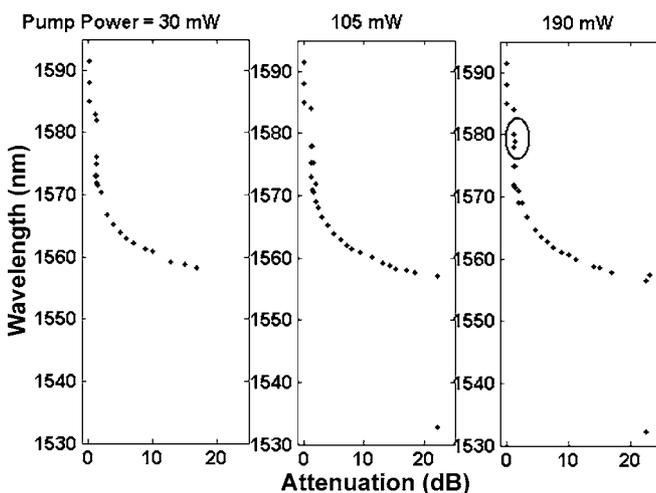
**FIGURE 6** Lasing wavelength at different values of  $\alpha$  for different pump powers with  $L = 4.6$  m,  $R = 0.99$
