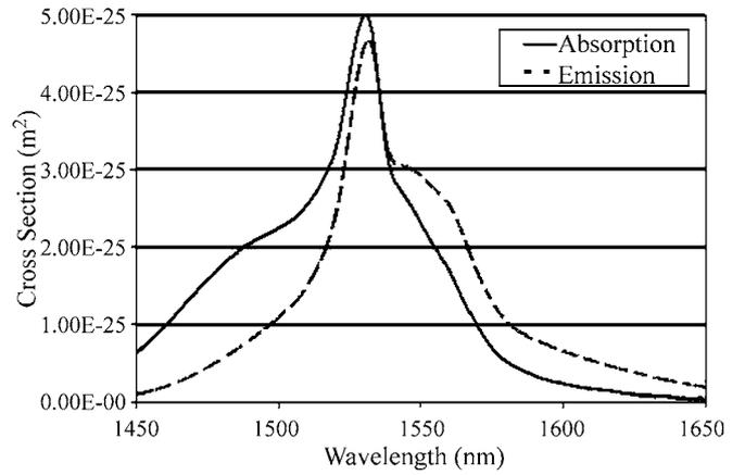
FIGURE 2 Emission and absorption cross-sections of the fiber studied
