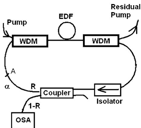
**FIGURE 1** Schematic of the erbium-doped fiber ring laser. ‘A’ indicates the position for the inclusion of optical attenuator which introduces a loss ( $\alpha$ )
