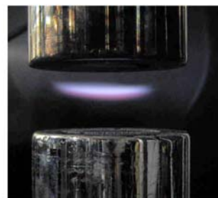
c Non-premixed hydrogen-air flame within a counter-flow burner
