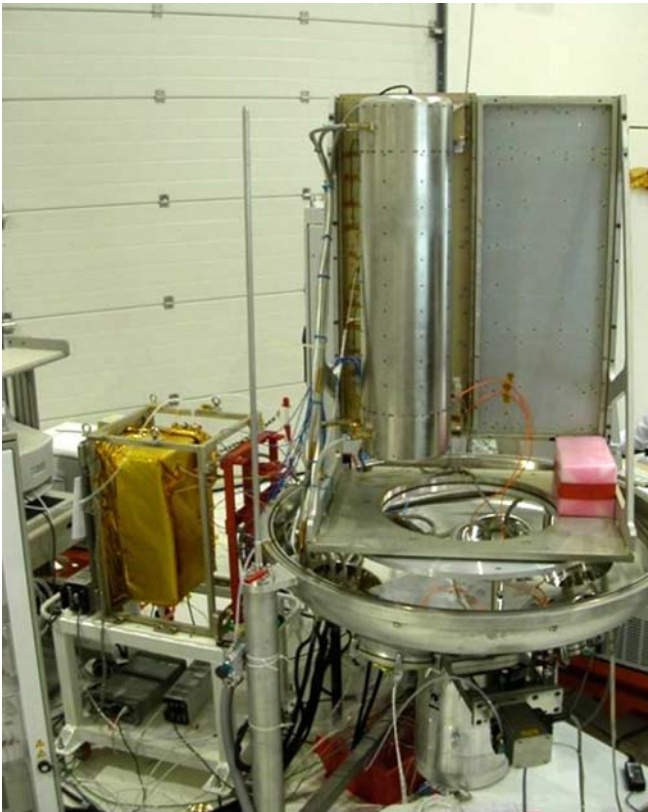
FIGURE 11 The PHARAO space clock under test in CNES, Toulouse. On Earth the tube is set vertical. The laser source (on the left) is covered with a multilayer insulator. In this picture the chamber in which the vacuum tests are performed is opened. The clock can be operated both at atmospheric pressure and in vacuum
