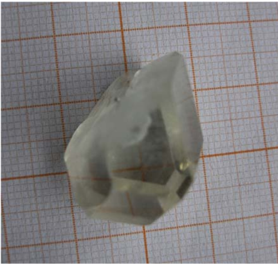
FIGURE 1 The as-grown crystal of \text{Yb}^{3+} :GAB
