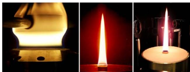
FIGURE 14 Target flames: modified McKenna (left), Gülder (center), Santoro (right). Operating conditions and measurement positions are given in Table 7
