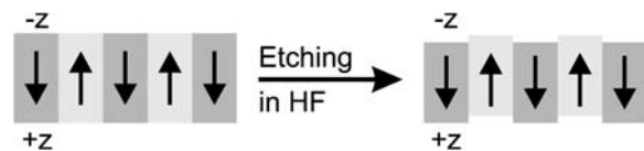
FIGURE 4 Selective etching for the visualization of antiparallel ferroelectric domains in z -cut LiNbO 3 , where the - z face etches much faster in hydrofluoric acid (HF) than the + z face, for which the etch rate is unmeasurably small
