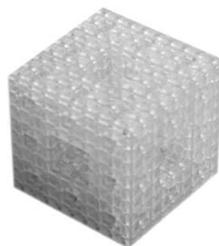
FIGURE 1 The Menger sponge fabricated by the stereolithography with a photoreactive epoxy resin as a raw material
