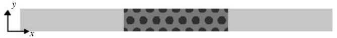
FIGURE 1 Schematic diagram of a heterogeneous layer in a two-dimensional photonic crystal. The system is infinitely periodic in the y direction
