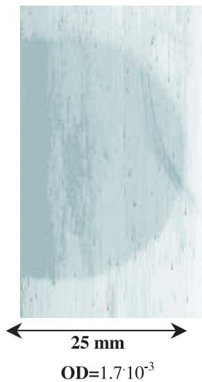
FIGURE 13 Copper layer spot deposited on a glass plate placed 6.5 cm from the plasma after being exposed to 1000 laser shots at I_L = 10^{10} W/cm 2 on the Cu target using the Debris Mitigation System (DMS). The first chopper disk was 2 cm from the plasma and the Kr pressure was 2.5 mbar. The glass optical density on the spot, compared with a non-exposed glass, was OD = 1.7 \times 10^{-3}
