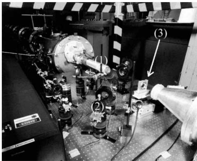
FIGURE 11 Picture of the HOLONS experiment. To the left the argon-ion laser for recording the gratings and to the lower right the evacuated tube for the detection system can be seen. (1) marks the end of the neutron-collimation system, (2) the beam expansion for the recording beams, (3) the photo-neutronrefractive sample (d-PMMA). Photograph by courtesy of GKSS
