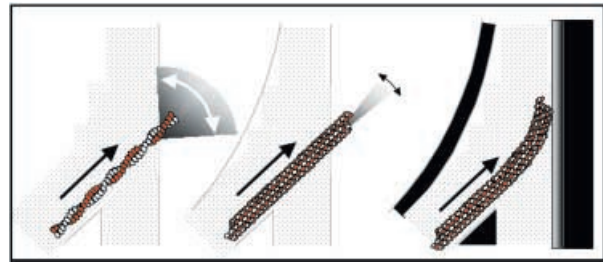
FIGURE 4 Left: An actin filament advancing over the boundary of a track of motor proteins will begin to swivel with the free tip and reach for the next available motor. Center: A microtubule in the same situation will swivel only slightly due to its 300-times-greater flexural rigidity. Right: Guiding channels with high sidewalls can force the microtubule into a turn provided the motors push the microtubule from behind
