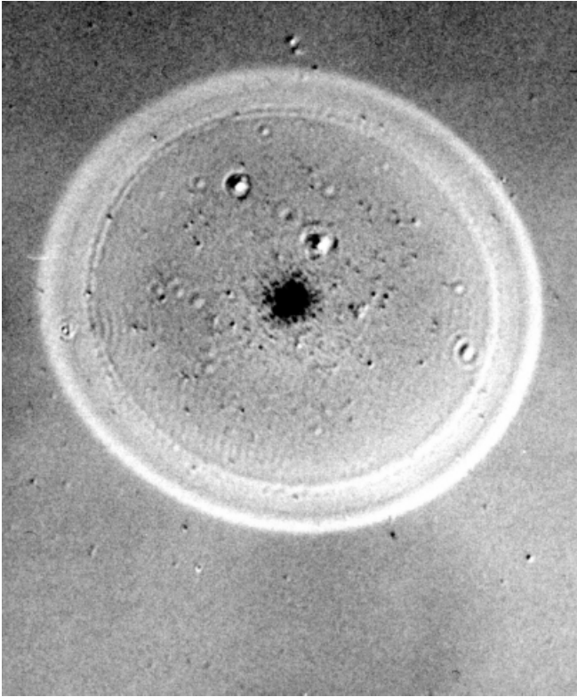
Fig. 2. Nomarski optical micrograph of the silicon sample surface treated with a single laser pulse in air ( \lambda = 800 nm, \tau = 130 fs, \Phi_0 = 1.5 J/cm 2 ). The outermost ring has a diameter of 45 \mu m
