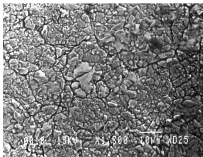
Fig. 3. Microstructure of the sintered samples ( x = 15 ). The micrograph is taken from a sample cut parallel to the pressing direction. Note the presence of lines corresponding to the cleavage planes
