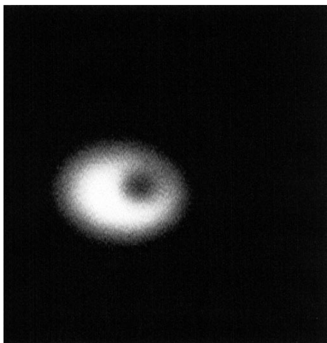
Fig. 5. Field-emission pattern from an open MWNT. V_T = -220 V
