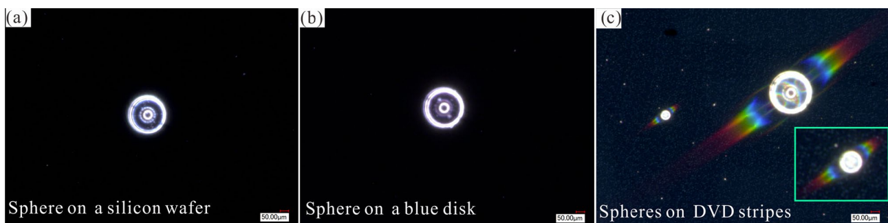
Fig. 2 The images of microspheres on three kinds of substrates. a A bigger size (180~212 μm) of BaTiO 3 microsphere on a silicon wafer, b the bigger size of BaTiO 3 microsphere on a Blu-ray disk, and c
