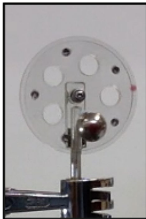
Fig. 17 Image of setup used to characterise moment of inertia of pulleys, by attaching a weight of known mass
