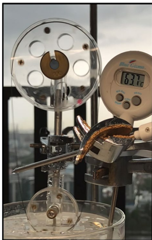
Fig. 13 Image of setup used to obtain energy curves: circular weights are attached to the centre of the top pulley
