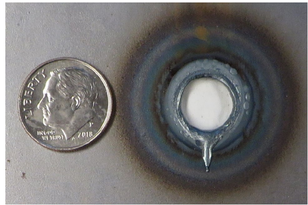
Fig. 6 A photograph taken with a Canon PowerShot digital camera shows a front view of the neck below the rim of a 9.88-mm-diameter hole in a 1.5-mm-thick steel plate, showing molten liquid draining preferentially at the front face of the sheet. A US dime (10-cent coin) is included for size comparison
