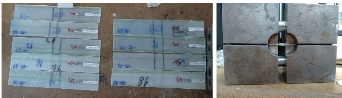
Fig. 3 Compression test specimens, standard clamping apparatus
