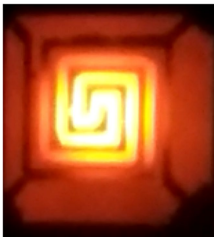
Fig. 7 Thermal stability testing: a microheater resistance versus testing time at different applied voltages, b optical image of heater glow before breakage and c SEM image of damaged structure
