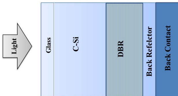
Fig. 1 Schematic of the proposed hybrid structure composed of front contact, active layer, DBR, back reflector and contact which are indium tin oxide (ITO) layer, c-Si, DBR and aluminum (Al), respectively
