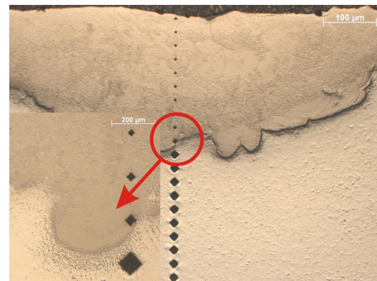
Fig. 12 Vickers microhardness imprints along the cross section of alloyed layer
