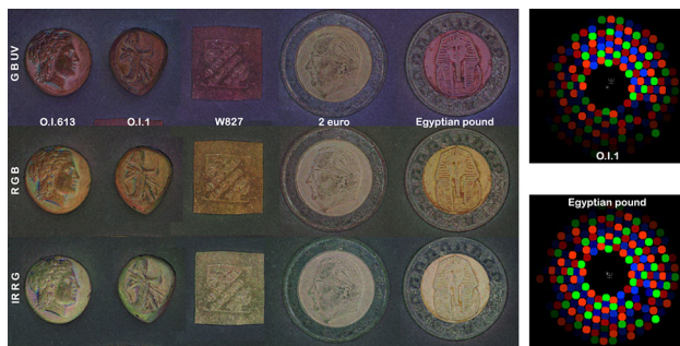
Fig. 8 False colour representations and 2 examples of spectral reflectance responses on the collection of coins (MS PLD, © ESAT-VISICS, KU Leuven)
