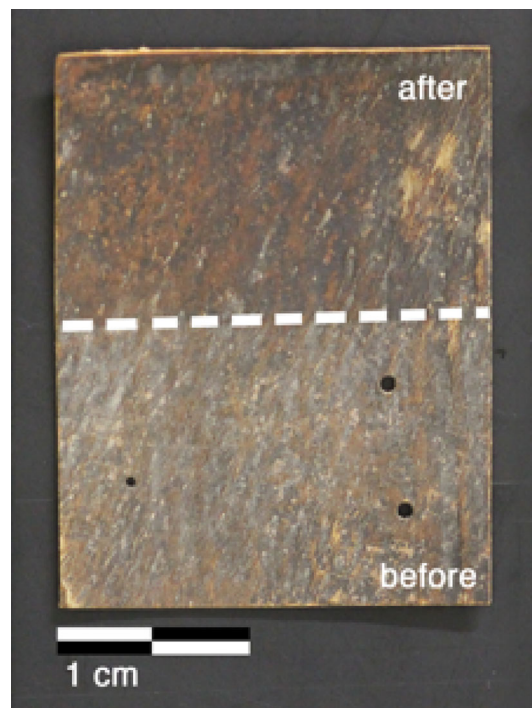
Fig. 6 H1 sample (Luther Bible cover, 1749 AD) before ( bottom ) and after ( top ) treatment with the pHEMA/PVP H58 gel (loaded with EAPC) and a mixed calcium hydroxide–calcium lactate nanoparticles dispersion in 2-propanol. The area on the bottom shows the dull grayish surface patina of dirt, salts, and pollutants. The area on the top shows the removal of the patina to reveal the underlying heterogeneous leather surface
