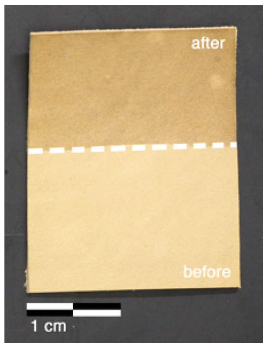
Fig. 3 M1 sample (modern leather, vegetable tanned, 10 cm × 15 cm) before ( bottom ) and after ( top ) treatment with a H58 gel (loaded with EAPC) and a mixed calcium hydroxide–calcium lactate nanoparticles dispersion in 2-propanol
